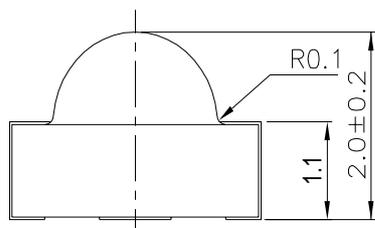
For reflow soldering (propose)
