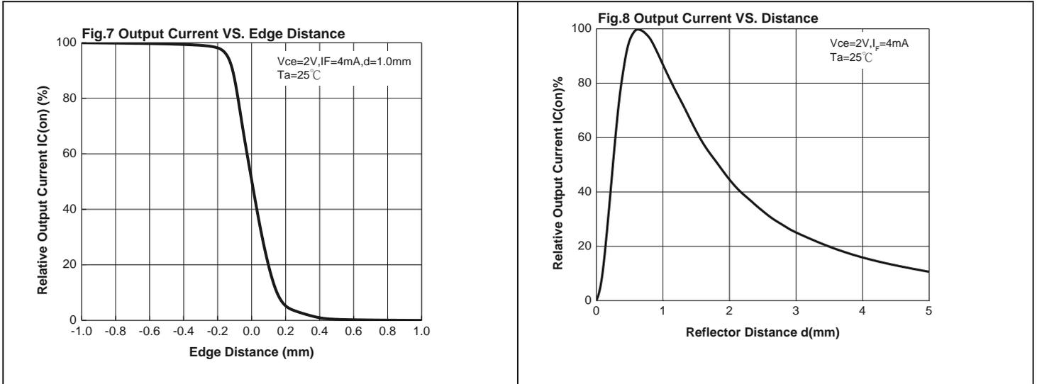
**Measuring Specification For Reflector Response**
